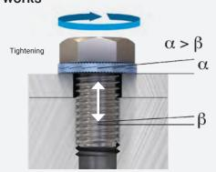
When the fastener is tightened, the cams lock and the serrations on the outer faces of the washers grip into both the fastener and the clamped part, creating clear impression marks in both. Clamping load has been created by the bolt, keeping the assembly locked in place.
